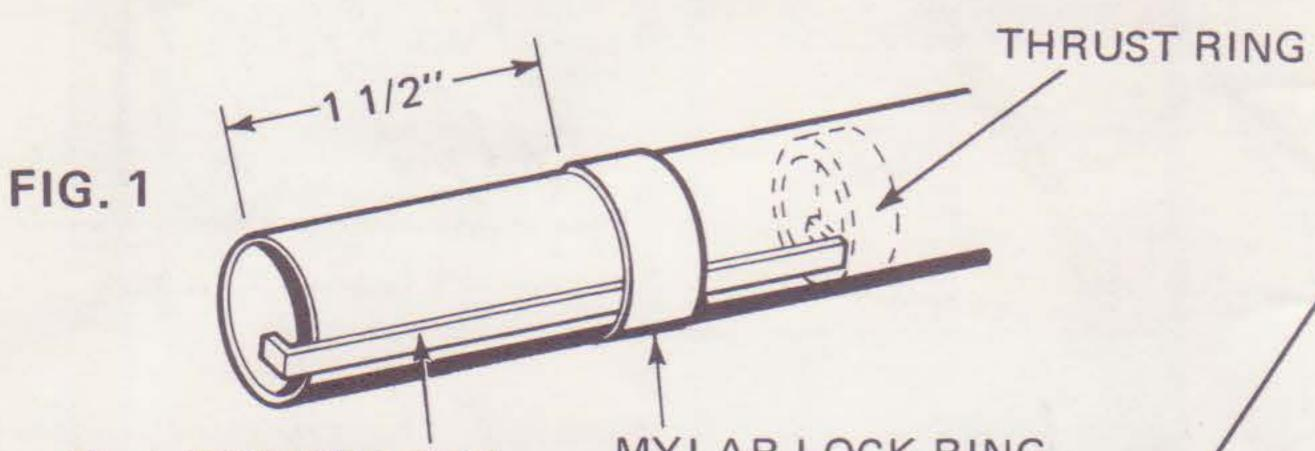
EL-1 ENGINE LOCK MYLAR LOCK RING
