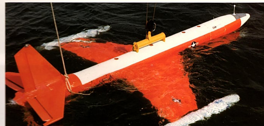
A sealed equipment bay permits water recoveries.
