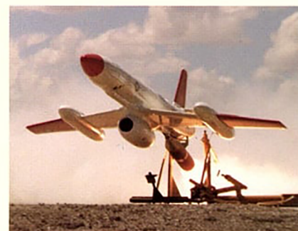
The MQM-107B can be rocket launched from the ground under adverse wind conditions including 50 kt headwinds, 20 kt crosswinds or tailwinds of 25 kt.
