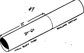
8.() Using the JT-60 as a back up for the mark, cut the tube as you did with the BT-20 in step #1. DO NOT CUT THROUGH THE JT-60. The long tube is the main body tube. The short will be the payload.
