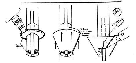
1.( ) Take the BT-50 and mark it at the 1 1/4", 2 1/2", and the 6 1/2" points. Cut a slot for the engine hook at the 2 1/2" mark. Install the hook.
