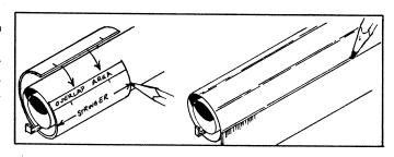
5.[\_] Measure and mark along the launch lug line 3". Run a bead of glue the length of the launch lug, and attach it along its line BELOW this mark.
