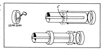
$3 \cdot [\_]$  Run a bead of glue inside one end of the BT-50 Main Body Tube. Slide the engine mount into the body tube until the thrust ends of each tube are flush. Let dry.
