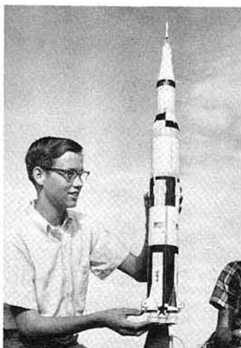
The Centuri Saturn 5 can be converted to Enerjet Power for single engine reliability. Since the simul-launch will be at night . . . you may suggest that a light of some kind be used for tracking.
