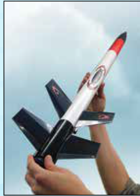
Ascender with booster flown on two F-15s, 99 N-SEC total impulse 7 second burn time.
