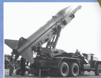
An iconic weapon of the Cold War, the MGR-1 Honest John battlefield rocket could carry nuclear or conventional warheads.
