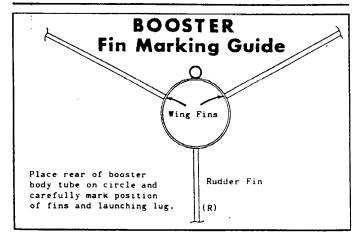
Use the booster fin guide (shown above) to mark the booster body tube. Three fins are used, and they must be placed in the correct relationship to the others in order to make the booster glide. The small fin is the rudder. Place a small "R" by your mark on the body tube for this fin so there will be no confusion
