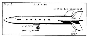
7. Apply glue to the root edges of the upper tip fins and position them on the topside of the main fins on the location marks. Glue the center fin into place on top of the launching lug, positioning it as shown in Fig. 3 and Fig. 5. Apply glue to the root edges of the lower tip fins and place them on the lower side of the main fin directly under the upper tip fins as shown in Fig. 3. Allow to dry.
