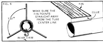
Spread glue on the root edge of one of the main fin pieces and position it on one of the guide lines. should stick straight away from the body tube as seen in the rear view. Repeat this step with the other two main fin pieces. Stand the bird on its nose while the main fins are drying.
