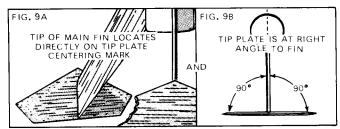
plate is resting flat on the table top. Repeat this step with the other two plates and fins. Stand the bird aside to dry.
