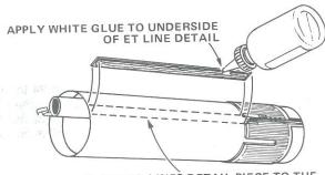
GLUE THE LINES DETAIL PIECE TO THE ET TUBE USING THE ALIGNMENT LINES
