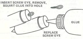
9 Insert the screw eye (part J) into the base of the nose cone (part K). Remove screw eye and squirt a small amount of glue into the hole. Re-insert the screw eye.
