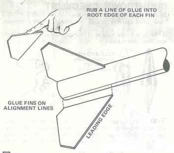
Rub a line of glue into the root edge of each fin and allow to dry. Glue the fins to the body on the fin alignment lines drawn in step 6. Refer to the illustration to be sure you position the fins correctly. Adjust the fins so they project straight away from the body tube. Do not set the rocket on its fins while the glue is wet.
