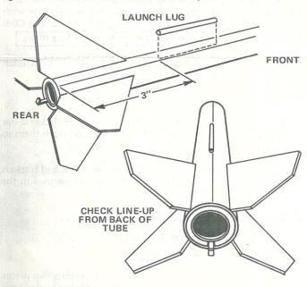
10 Glue the launch lug (part L) to the body on its line. The rear of the lug should be 3" from the rear of the body. Align it straight on the body.
