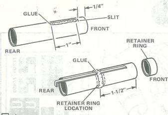
1 Cut a 1/8" long slit in the engine mount tube (part A), 1/4" from one end as shown. Apply a 1" long line of glue to the tube as shown. Push one end of the engine hook (part B) into the slit and press the main part of the hook into the glue. Apply a line of glue around the middle of the tube and slide the retainer ring (part C) over tube and hook onto the glue.
