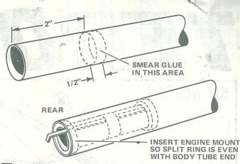
5 Smear glue around the inside of the other end of the body tube to cover an area about 2" to 2-1/2" from the end of the tube. Immediately insert the engine mount unit, being careful to position it so the engine hook will stick out of the end of the tube. Push the engine mount in with one smooth motion until the ends of the tubes (and the split ring) are even.
