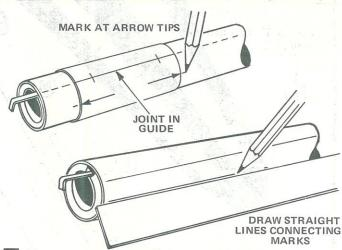
Cut out the body tube marking guide from the pattern sheet. Wrap it around the rear of the body so the joint in the guide is in line with the engine hook. Mark the tube at each arrow point, front and rear. Draw a straight line connecting each matching front and rear mark. (Use a ruler when drawing lines.) Extend the launch lug line forward 5".
