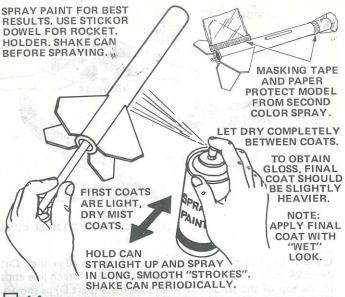
14 After the sanding sealer is completely dry, paint the entire model white. Let the white dry overnight. Apply masking tape and paper to cover and protect the areas which will remain white. (See the Decor Layout illustration.) paint three fins and the exposed body red. Carefully remove the masking tape and paper as soon as the paint is dry.
