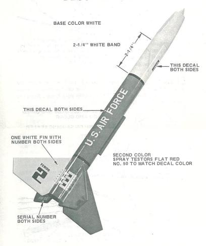
15 When all paint is dry, apply decals (part P). Peel a decal section from the backing, dip it in mildly soapy water, and position it on the model. Blot excess water away. For best results, let the model dry overnight and apply a coat of clear spray to protect paint and decals.
