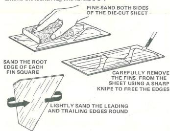
**7** Fine-sand the balsa sheet (part I), then carefully remove the die-cut fins from the sheet. Free the edges with a sharp knife. Sand the leading and trailing edges of the fins round. Leave the root edge square.
