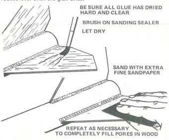
13 When all glue on the outside of the body is dry, prepare the fins for painting. Apply at least two coats of sanding sealer to the fins. Let dry and sand lightly between coats. Do this until the tiny holes in the wood are filled and everything looks and feels smooth. For best results let the model dry overnight.
