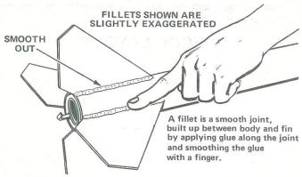
12 Apply a glue "fillet" to each fin joint. Holding the rocket horizontally (level), apply a line of glue to both sides of each joint. Smooth out the glue with your finger. Keep the rocket level until the glue dries.
