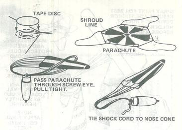
11 Cut out the parachute (part M) on its edge lines. Cut three 24 inch lengths of shroud line (part N). Attach line ends to the top of the parachute with tape discs (part O) as shown. Pass the shroud line loops through the screw eye at the rear of the nose cone. Pass the parachute through the loop ends and draw line tight against the screw eye. Set the knot with a drop of glue. Tie the free end of the shock cord to the screw eye.
