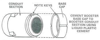
Remove the booster base cap from the plastic parts set (part F). Using the molded keyways for positioning, glue together the booster conduit section and the base cap. Use liquid plastic cement. Set aside to dry.
