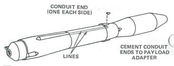
16 Cut the small conduit ends from the plastic parts set. Trim any flash from their edges. Use liquid plastic cement to cement these to the payload adapter as shown. They should be positioned so that they are centered between the conduit lines drawn on the 3rd stage body tube.
