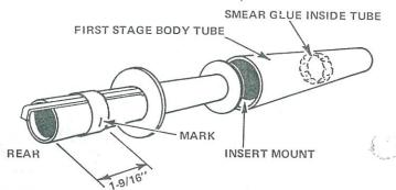
Mark the engine mount tube 1-9/16" from the engine hook end. Smear glue around the inside of one end of the 1st
