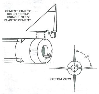
15 Cut the fins from the plastic parts set. Carefully trim any flash from their edges. Use liquid plastic cement to cement the fins to the booster base cap. Note that the molded keys on the fins fit into the molded grooves in the booster base cap. Check alignment frequently while the cement is setting.
