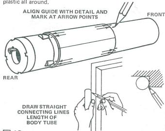
12 Cut out the 1st stage marking guide from the pattern sheet. Wrap it around the first stage booster tube, making sure the set of arrows lines up with the detail on the booster conduit section. Mark the tube at each arrow point. Carefully connect each pair of arrow points with a straight line drawn the length of the tube as shown.
