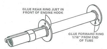
2 Separate the adapter rings (part C) from the die-cut card. Slide one ring onto the tube from the forward end. Place it just in front of the engine hook. Slide the other ring into place 1/16" from the forward end of the tube. Apply a line of glue at the ring/tube joint on both sides of each ring. Let the assembly dry completely.
