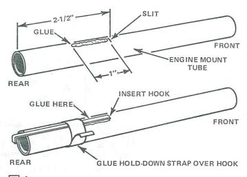
Mark the engine mount tube (part A) 2-1/2" from one end. Cut a 1/8" long slit in the tube at the mark as shown. Cut out the hold-down strap from the pattern sheet (part R). Apply a 1" long line of glue to the tube as shown. Push one end of the engine hook (part B) into the slit and press the main part of the hook into the glue. Apply glue to one side of the hold-down strap and wrap it tightly around the middle of the tube over the engine hook.
