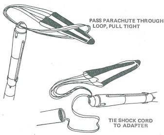
24 Cut out the parachute (part M) on its edge lines. Cut three 36" lengths of shroud line (part N). Attach the line ends to the top of the parachute with tape discs (part O) as shown. Pass the shroud line loops through the molded eyelet in the third stage adapter. Pass the parachute through the loop ends and draw the lines tight against the eyelet. Set the knot with a drop of glue. Tie the free end of the shock cord to the eyelet.
