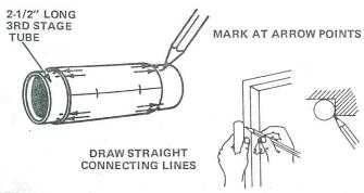
Cut out the 3rd stage marking guide from the pattern sheet. Wrap it around the 2-1/2" long 3rd stage body tube (part I). Mark the tube at each of the arrow points with a pencil. Draw straight lines the length of the tube connecting the matching pairs of conduit marks. Mark the payload end and the 3rd stage adapter end of the tube.
