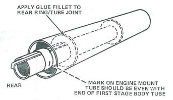
stage body tube (part D) as far in as possible (but not more than 4-1/2"). Immediately insert the engine mount assembly. Push it in with one smooth motion until the mark on the engine mount tube is even with the rear of the tube. Apply a line of glue to the joint between the rear ring and the body tube. Set the tube on its forward end while the glue dries.
