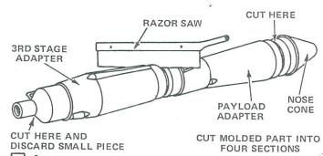
Cut the molded nose cone piece (part G) into four sections in the same manner as the molded adapter piece. The four pieces are the nose cone, the payload adapter, the 3rd stage adapter, and the end piece which is discarded. Cut off any molding flash from the shock cord eyelet and from the base of the 3rd stage adapter.
