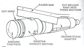
If you have a razor saw, use it to cut the molded adapter piece (part E) into three parts as shown. If you do not have a razor saw, use a model knife or single edge razor blade. Make very light cuts around the parting lines (bottom of grooves) and repeat until you have cut completely through the plastic. Work carefully to avoid tearing the plastic. One piece is the booster conduit section, one piece is the second stage adapter, and the short conical section is to be discarded.
