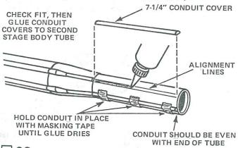
20 Test fit the 7-1/4" long conduit covers on the second stage body tube. Position the covers between the lines drawn on the tube and with one end just touching the molded detail on the second stage adapter. Apply a line of glue along the body tube between one set of lines and press one of the conduit covers in place, checking for proper alignment. Hold it in place with small strips of masking tape as shown. Repeat this with the other 7-1/4" long conduit cover.
