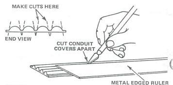
18 Use a metal edged ruler as a guide to cut the conduit covers (part K) apart as shown. If necessary, sand the edges of
