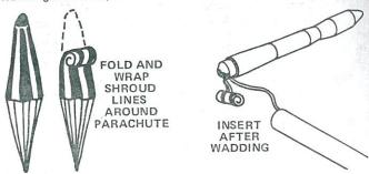
T-13 Fold the parachute into a triangular shape. Roll 'chute tightly as shown and wrap shroud lines around it. Slide 'chute into body above wadding. If 'chute is too large, unroll and repack until it slides easily into rocket. A fit that is too tight may prevent parachute from ejecting properly.
