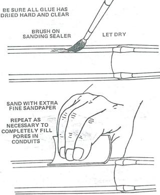
26 Apply two or more coats of sanding sealer to the conduit cover surfaces. Sand lightly with extra fine sandpaper between coats. Repeat until the surfaces look and feel smooth. Apply additional sanding sealer to all conduit edges where they touch the body tubes to seal any gaps that may still exist. Sand smooth.
