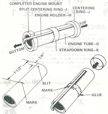
Locate the parts called out in the illustration above. Cut a 1/8" wide slit, 1/4" from the end of the tube and place a mark on the tube 1-1/2" from same end. Run a bead of glue from slit to mark. Place one end of engine holder in slit. Hold engine holder in place and run a bead of glue around tube above mark. Slide strapdown ring over top of tube and push down to mark. Glue centering ring to top and split ring to bottom of tube, flush with the ends.
