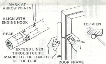
Cut out the body tube marking guide from the pattern sheet. Wrap it around the rear of the body so the launch lug marks are in line with the engine hook. Mark the tube at each arrow point, front and rear. Draw a straight line connecting each matching front and rear mark. (Use a door frame as a guide when drawing lines). Extend the lines to the middle of the tube.
