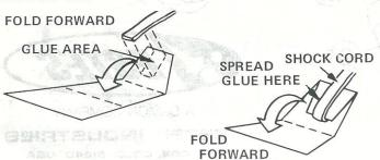
Crease it on the dotted lines by folding. Spread glue on the first section (1) and lay the end of the shock cord (part N) into the glue. Fold over and apply glue to the back of the first section and the exposed part of section 2. Lay the shock cord as shown and fold over again. Clamp the unit together with you fingers until the glue sets.
