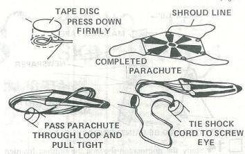
11 Cut out the parachute (part M) on its edge lines. Cut three 24" lengths of shroud line (part O). Attach line ends to the top of the parachute with tape discs (part P) as shown. Pass the shroud line loops through the screw eye on the payload section. Pass the parachute through the loop ends and pull the lines tight against the screw eye. Set the knot with a drop of glue. Tie the free end of the shock cord to the screw eye.
