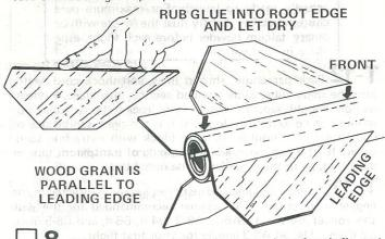
Rub a line of glue into the root edge of each fin and allow to dry. Glue the fins to the body on the fin alignment lines drawn in step 6. Refer to the illustration to be sure you position the fins correctly. Adjust the fins so they project straight away from the body tube. Do not set the rocket on its fins while the glue is wet.
