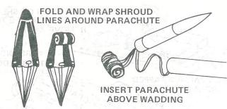
**T-13** Fold the parachute into a triangular shape. Roll the 'chute tightly as shown and wrap the shroud lines around it. If 'chute is too large, unroll it and repack until it slides easily into rocket. A fit that is too tight may prevent the parachute from ejecting properly.
