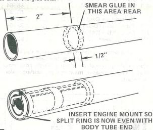
5 Smear glue around the inside of the rear end of the main body tube (the end <u>away</u> from the shock cord mount). The glue should cover an area about 2" to 2-1/2" from the end of the tube. Push the engine mount unit in right away--but be sure the mount is turned so the hook will stick out of the end of the tube! Push the engine mount in with one smooth motion until the ends of the tubes (and the split ring) are even.
