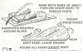
7 Fine-sand the balsa sheet (part C), then carefully remove the fins from the sheet. Free the edges with a sharp knife. Sand all edges except the root edge to a rounded shape. Make sure the root edge stays square.
