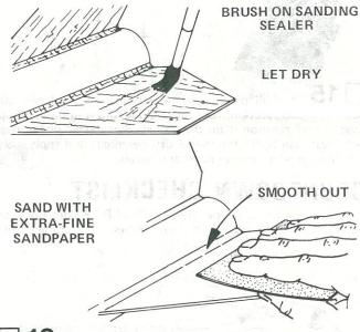
13 When all glue on the outside of the body is dry, prepare the fins for painting. Apply at least two coats of sanding sealer to the fins. Let dry and sand thoroughly between coats. Do this until the tiny holes in the wood are filled and everything looks and feels smooth. Install the nose cone (part D) in the front of the payload section. Paint the entire rocket gloss white. Let the paint dry overnight.
