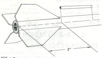
10 Glue the launch lug (part F) to the body on its line. The rear of the lug should be 3" from the rear of the body. Align the lug straight on the body.
