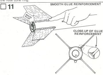
Apply a glue reinforcement to each fin joint and launch lug. Holding the model level, apply a line of glue to both sides of each joint. Smooth out the glue with your finger. Keep the model level until the glue dries.
