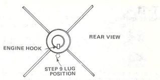
Apply glue to the root edge of one fin. Glue fin to the fin alignment line so rear of fin is even with the end of the body tube. Be sure fin projects straight out from the body tube. Allow to dry. Repeat for the remaining fins.
