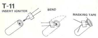
Select an engine and install an igniter as directed in the engine instructions. Use an A8-3 engine for your first flight.
