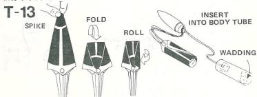
Hold the parachute at its center and pass the other hand down it to form a "spike" shape. Fold this spike in half. Roll parachute into tube shape to fit easily into body. Pack 'chute into the tube on top of the wadding. Pack the shroud lines and shock cord in on top of the parachute and slip the nose cone into place.
