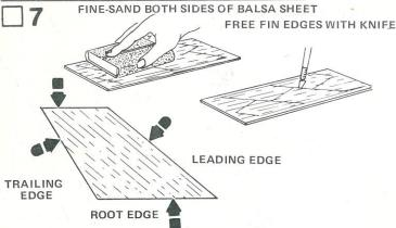
Fine-sand the balsa sheets (part K), then carefully remove the diecut fins from the sheet. Free the edges with a sharp knife. Sand the leading and trailing edges of the fins round. Leave the other edges square.
