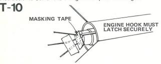
Insert engine into rocket engine mount. Engine hook must latch securely over end of the engine.
