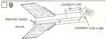
Glue the launch lug (part E) to the body on its line. The front of the lug should be 8" from the rear of the body. Align it straight on the body.
