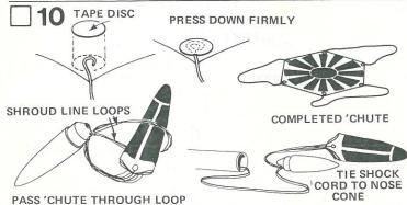
Cut out the parachute (part J) on its edge lines. Cut three 36" lengths of shroud line (part H). Attach line ends to the top of the parachute with tape discs (part I) as shown. Pass the shroud line loops through the ring on the nose cone (part F). Pass the parachute through the loop ends and draw the lines tight against the ring. Set the knot with a drop of glue. Tie the free end of the shock cord to the nose cone ring.
