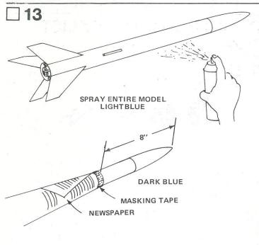
Spray paint the entire rocket with light blue spray enamel. When this is dry, measure 8" from the tip of the nose cone down the body tube and place a mark. Wrap the remaining portion of the rocket with newspaper and seal with masking tape to prevent the paint from running under the paper. Spray paint the nose cone and body tube to the mark with dark blue spray enamel. When painting your rocket, spray several light "mist" coats of paint rather than one heavy coat.
