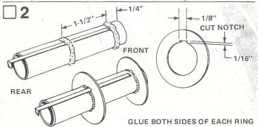
Separate the adapter rings from the die-cut card (part B). Cut a notch in one of the rings as illustrated and glue the rings to the engine mount tube. The notched ring should be placed over the engine hook. Let this assembly dry completely.
