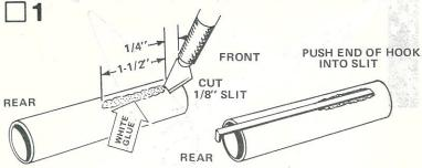
Cut a 1/8" wide slit in the engine mount tube (part A), 1/4" from one end as shown. Apply a 1-1/2" long line of glue to the tube as shown. Push one end of the engine hook (part C) into the slit and press the main part of the hook into the glue.
