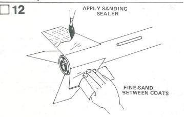
Apply all glue reinforcements to fins and launch lug as shown in Step 11. There will be ten reinforcements. Let all glue dry completely. Apply sanding sealer to all balsa surfaces. Allow the sealer to dry and sand it smooth. Repeat this step as many times as needed to fill all the grain lines in the wood. Use either dope or enamel to finish your model, but don't use one over the other.
