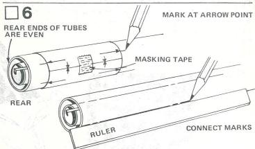
Cut out the body tube marking guide. Wrap it around the rear of the body tube. Mark the tube at each arrow point, front and rear. Draw a straight line connecting each matching front and rear mark. (Use a ruler when drawing lines.) Extend the launch lug line forward 8" (align launch lug line with engine hook).
