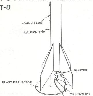
Slide launch rod through rocket launch lug and place rocket on launch pad. Make sure the rocket slides freely on the launch rod. Clean the micro-clips and attach them to the igniter wires. Arrange the clips so they do not touch each other or the metal blast deflector. Attach clips as close to engine as possible.
