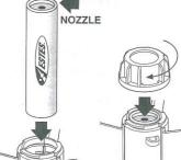
A. Remove engine cap. Insert engine.
