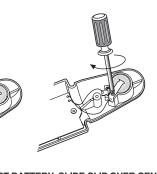
4. INSERT BATTERY. SLIDE CLIP OVER CENTER OF BATTERY. TIGHTEN SCREW.
