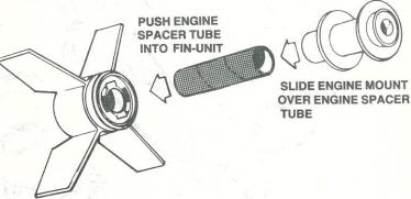
Make sure all glue joints on engine mount are dry. Test-fit the engine mount into the body tube (part F) by smoothly inserting and removing it. Sand if necessary to assure a smooth fit. Insert the plastic fin-unit (part G) into the lock ring (part H) and turn clockwise 1/4 turn or until fin-unit stops. Do not force or over tighten. Push engine spacer tube all the way into fin-unit and slide engine mount all the way down onto engine spacer tube.
