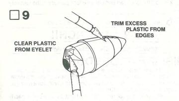
Trim or sand any excess plastic from around the sides of the nose cone (part J). Use a sharp knife to remove any excess plastic from the inside of the molded eyelet at the rear of the nose cone.
