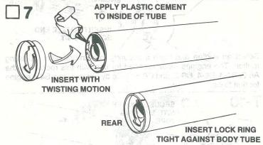
Remove the fin-unit from the lock ring by turning counter-clockwise. Apply a line of tube-type plastic cement around the inside rear of the body tube. Slide the lock ring into the end of the tube and twist it as it is pushed into place. Be sure it is inserted all the way. Stand rocket body vertically on the lock ring and allow cement to dry. Do not put fin-unit into lock ring until cement is completely dry.
