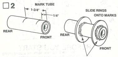
APPLY GLUE TO JOINT ON BOTH SIDES
