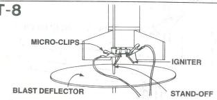
Slide the launch rod through rocket launch lug. Make sure the rocket slides freely on the launch rod. The rocket must be supported by a "stand-off" to keep the igniter wires from touching the metal blast deflector. If your launch system does not have a stand-off, wrap a piece of masking around the launch rod to support the rocket. Clean the micro-clips and attach them to the igniter wires. Arrange the clips so they do not touch each other or the metal blast deflector.
