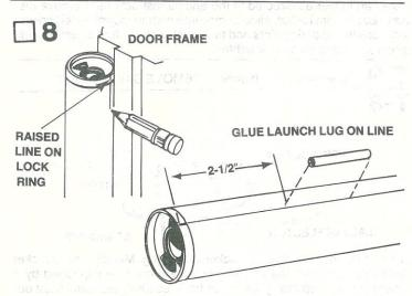
Locate raised line on side of lock ring. Draw a straight line from this raised line down the length of the body tube. A door frame inside edge can be used as a guide. Make sure line is straight along tube. Glue launch lug (part I) to rocket body tube 2-1/2" from the rear of the lock ring. Align the launch lug straight along tube.
