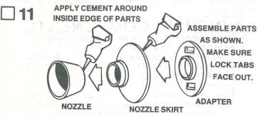
Locate the plastic display nozzle parts (part N). Carefully trim away the small projections where the parts were connected to the molding sprue. Assemble the plastic components using tube-type plastic cement. Set aside to dry.
