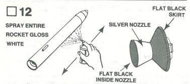
After the glue and cement is dry on model, paint entire model gloss white. You may, if you wish, mask off fins so fins remain clear and paint fin-unit white also, or you can leave fin-unit clear and not paint it. We recommend spray enamel. Do not paint the model with lacquer paint. Follow instructions on spray can for best results. Paint display nozzle as shown.
