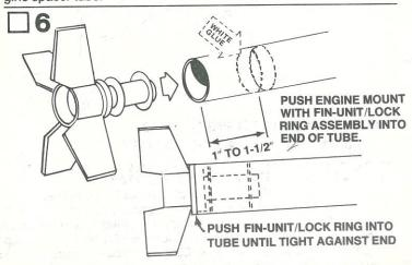
Test-fit the complete fin-unit and engine mount assembly into the body tube to see how the assembly fits. Remove fin-unit and engine mount
