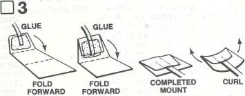
Cut out the shock cord mount from the front of the instruction sheet. Fold it on the dotted lines. Spread glue on the first section (1) and lay the end of the shock cord (part E) into the glue. Fold over and apply glue to the back of the first section and the exposed part of section 2. Lay the shock cord as shown and fold over again. Clamp the unit together with your fingers until the glue sets.
