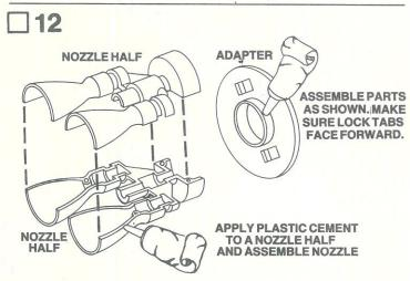
Locate plastic display nozzle parts from the plastic parts set. Carefully trim away the small projections where the parts were connected to the molding sprue. Assemble the parts using tube-type plastic cement. Set aside to dry.
