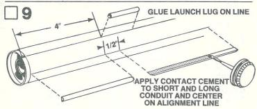
Glue the launch lug (part I) to rocket body tube on line drawn up from raised line on lock ring. The rear of the launch lug should be 4" from the rear of the lock ring. Align the launch lug straight with the body tube. Apply contact cement to the flat side of the plastic conduits from plastic parts (part J). Align them on their alignment line as shown. Wipe away any excess cement and set aside to dry.
