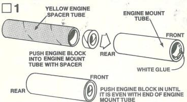
Apply glue around the inside of one end of the engine mount tube (part A) about 3/16" from the end of the tube. Immediately slide the engine block (part B) into the opposite end of the tube and push engine block up even with end of engine mount tube with the yellow engine spacer tube (part C). Immediately remove spacer tube and wipe away any excess glue from front of tube.
