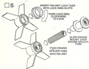
Make sure all glue joints on engine mount are dry. Test-fit the engine mount into the body tube (part F) by smoothly inserting and removing it. Sand if necessary to assure a smooth fit. Insert the plastic fin-unit (part G) into the lock ring (part H) and turn clockwise 1/4 turn or until fin-unit stops. Do not force or over tighten. Push engine spacer tube all the way into fin-unit and slide engine mount all the way down onto engine spacer tube.
