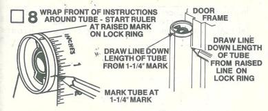
Mark body tube 1-1/4" from raised line on side of lock ring as shown with ruler printed on front of instruction sheet. Draw straight lines from the raised line and the 1-1/4" mark down the length of the tube. A door frame inside edge can be used as a guide as shown. Make sure these lines are straight along tube.
