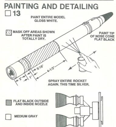
After glue and cement are dry on model, paint entire model gloss white. After paint is thoroughly dry, mask off areas shown and paint model silver. You may, if you wish, mask off fins so fins remain clear and paint fin-unit silver also. We recommend spray enamel for best results. Do not paint the model with lacquer paint. Follow instructions on spray can for best results. Paint display nozzles as shown.
