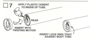
Remove the fin-unit from the lock ring by turning counter-clockwise. Apply a line of tube-type plastic cement around the inside rear of the body tube. Slide the lock ring into the end of the body tube and twist it as it is pushed into place. Be sure it is inserted all the way. Stand rocket body vertically on the lock ring and allow cement to dry. Do not put fin-unit into lock ring until cement is completely dry.
