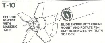
Install an igniter as directed in the engine instructions. Remove display nozzle from rocket, slide engine into engine mount. Insert fin-unit lock tabs into lock ring slots and turn clockwise 1/4 turn or until fin-unit stops. Do not force or over tighten.
