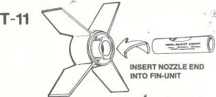
Select an engine and push it securely into fin-unit with a twisting motion. The engines recommended for use with this rocket are the A8-3, B4-4, B6-4, C6-3, and C6-5 made by Estes. Use a B4-4 engine for first flight.
