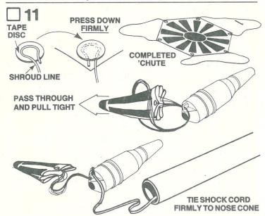
Cut out the parachute (part L) on its edge lines. Cut three equal lengths of shroud line (part M). Attach line ends to the top of the parachute with tape discs (part N) as shown. Form a small loop in the
