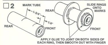
Mark the engine mount tube at 1/4" and 1-3/4" from the front (end with engine block). Carefully remove the two adapter rings from the die-cut card (part D). Use a sharp knife to free the rings from the card. Slide rings onto the tube so one is at each mark. Apply a line of glue around both sides of rings where it touches the tube. Smooth out glue with finger. Set the assembly aside to dry.
