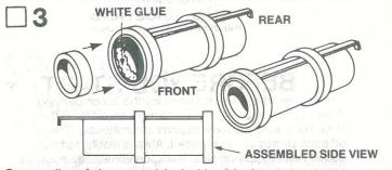
Smear a line of glue around the inside of the forward end of the engine mount tube and push the engine block (part D) in until it stops against the engine hook. Set the unit aside to dry.
