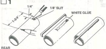
Mark the engine mount tube (part A) 1/4" and 1-3/4" from one end. Cut a 1/8" long slit in the tube at the 1/4" mark. Apply a line of glue between the two marks. Push one end of the engine hook (part B) into the slit as shown. Press the main part of the hook into the glue.
