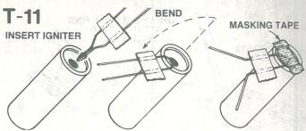
Select an engine and install an igniter as directed in the engine instructions. Use a D12-5 engine only.
