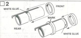
Apply a line of glue around the tube just forward of the 1-3/4" mark. Slide one of the adapter rings (part C) onto the tube from the forward end, over the engine hook, and up to the 1-3/4" mark. Apply a line of glue around the tube just forward of the engine hook. Slide the remaining adapter ring onto the forward end of the tube until it just touches the engine hook.
