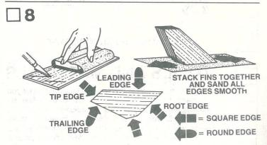
Fine-sand the balsa die-cut sheet (part H), then carefully remove the die-cut fins from the sheet. Free the edges with a sharp knife. Sand the leading and trailing edges of the fins round. Leave other edges square.
