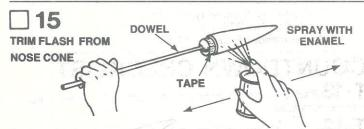
Spray paint the nose cone (part J) with several light coats of flat blue paint. The nose cone can be supported by a dowel or stick inserted in the center opening in the nose cone while being painted and drying. A layer of masking tape around nose cone shoulder works well to protect the nose cone shoulder from "overspray" while painting.
