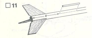
Glue launch lug (part I) to rocket body tube on the launch lug line. The rear of the launch lug should be 4" from the rear of the rocket body tube. Align the launch lug straight along the body.
