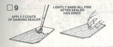
Apply a coat of sanding sealer to each fin. Apply sealer to all edges except the root edge. When sealer is dry, lightly sand all the sealed surfaces. Repeat sealing and sanding process until balsa grain no longer shows. Resand root edge, lightly, to remove any trace of sealer.
