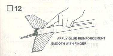
Apply glue reinforcements to each fin/body tube joint. Holding the model level, apply a narrow line of glue to both sides of each fin joint. Smooth out the glue with your finger. Apply glue reinforcement on both sides of launch lug. IMPORTANT—Keep the model level until the glue dries.
