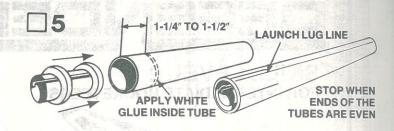
Smear a line of glue around the inside of the rear end of the body tube. The glue line should be about 1" to 1-1/2" from the end of the tube. Push the engine mount unit in right away -- but be sure the mount is turned so the hook will stick out of the end of the tube. Position the engine mount so that the engine hook is centered with the launch lug line. Push the engine mount in with one smooth motion until the ends of the tubes are even.
