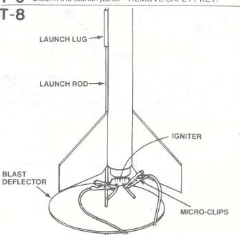
Slide launch rod through rocket launch lug and place rocket on launch pad. Make sure the rocket slides freely on the launch rod. Clean the micro-clips and attach them to the igniter wires. Arrange the clips so they do not touch each other or the metal blast deflector. Attach clips as close to protective tape on igniter as possible.
