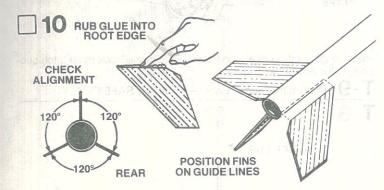
Rub a line of glue into the root edge of each fin and allow to dry. Apply glue to the fins and position fins on the alignment lines in their correct positions on the tube. Refer to the illustration to be sure of these positions. Adjust the fins so they project straight away from the body tube. Do not set the rocket on its fins while the glue is wet.
