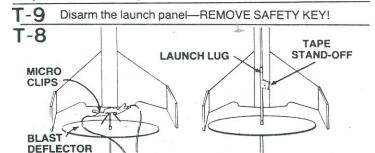
Slide launch rod through rocket launch lug and place rocket on launch pad. Make sure the rocket slides freely on the launch rod. Clean the micro-clips and attach them to the igniter wires. Arrange the clips so they do not touch each other or the metal blast deflector. Attach clips as close to protective tape on igniter as possible.
