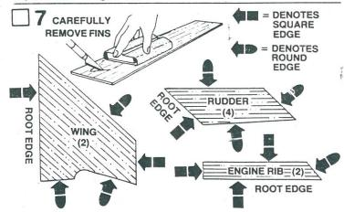
Fine-sand both sides of the balsa sheet (part G). Carefully remove the fins from the sheet using a sharp knife. Sand all fin edges. The root edge of each fin must be square.
