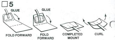
Cut out the shock cord mount from the middle of the tube marking guide. Crease it on the dotted lines by folding. Spread glue on the first section (1) and lay the end of the shock cord (part F) into the glue. Fold over and apply glue to the back of the first section and the exposed part of Section (2). Lay the shock cord as shown and fold over again. Clamp the unit together with your fingers until the glue sets.
