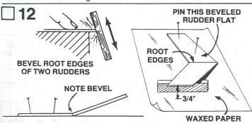
Ind a bevel into the root edges of two rudders. Lay a piece of waxed were on the work surface and pin down one of the beveled rudders. Do not damage the surface on which you are working. Rub glue into the root edge of one of the un-beveled rudders. Position the root edges of the two pieces tightly together. Raise the un-pinned rudder tip 3/4" as shown while the glue dries. Assemble the two remaining rudders in the same manner.
