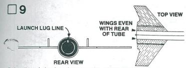
Rub a line of glue into the root edge of both wings and allow to dry. Glue the wings to the body tube on the alignment lines as shown. The rear of each wing should be even with the rear of the body tube as shown. Adjust the wings so that they project straight out from the body tube. Do not set the rocket on its wings while the glue is drying.
