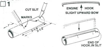
Mark the engine mount tube (part A) at 1", 2-1/4" and 2-1/2" from one end. Cut a 1/8" long slit at the 2-1/2" mark. Gently bend th engine hook (part B) so that it bows upward very slightly in the middle. (Study the drawing—Don't bend the wrong way.) Insert one end of the engine hook into the slit in the tube.
