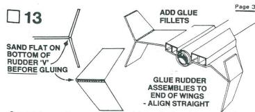
Sand flat a small area at the glue joint on both rudder assemblies as shown. This makes a better and stronger glue joint. rub a thin layer of glue onto these flat areas and allow to dry. Apply a line of glue to the end of a wing and press a rudder assembly into place. Check for straight alignment and allow the glue to dry. Repeat this with the other rudder assembly and wing. When all the glue is dry, add reinforcement fillets of glue as shown to all rudder-wing joints.
