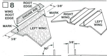
Using the illustration as a guide, lay out the parts to create two wings one left and one right. Mark both wings 3/8" in from the root edge both leading and trailing edges. Then use a ruler to draw a line connecting the marks. Rub a line of glue into the root edges of both Engine Ribs and allow to dry. Glue the Engine Ribs to the wings next to the lines as shown. Check to be sure the Ribs stand straight up before the glue dries.
