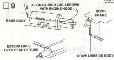
Cut the BT-50 marking guide from page 5 of the instructions. Wrap the guide around the rear of the body tube and tape the ends together. Rotate the guide so the launch lug arrow is lined up with the engine hook. Mark the location of the launch lug, rudder and wings. Remove the guide and draw lines from the rear of the tube forward about 3". Extend the lines over the rear of the tube so they will show when the parts are attached.
