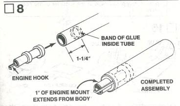
Use a small stick to apply a generous band of glue about 1-1/4" inside one end of the BT-50FE body tube (part I). Making sure the engine hook extends to the rear, slide the engine mount into the body tube. Without pausing, slide the engine mount forward until the rear ring is even with the rear of the body tube.
