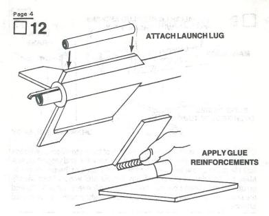
Glue the launch lug (part K) to the launch lug stand-off. As previously described, apply glue reinforcements to all joints. Support the model in a horizontal position until the glue dries.
