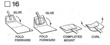
Cut out the shock cord mount from page 5 of the instructions. Fold on dotted lines, then unfold and apply glue to Section 1. Lay the end of the shock cord (part N) into the glue. Fold over and apply glue to the back of Section 1 and the exposed portion of Section 2. Fold again to complete mount. Curl the edges of the mount up so it will match the contour of the body tube and hold with your fingers until the glue sets.
