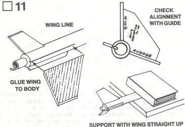
Cut the wing alignment guide from the back of the kit panel (part J). Apply glue to the root edge of a wing and attach it to the body. Use the guide to check wing-rudder alignment. Support the model with the wing pointing straight up. Re-check the alignment after a few minutes and make corrections if necessary. Leave the model undisturbed until the glue is completely dry. Attach the remaining wing in the same manner.
