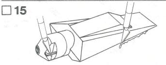
Trim or sand any excess plastic from around the sides of the nose cone (part M). Use a sharp knife to remove any excess plastic from the inside of the molded eyelet at the rear of the nose cone. Wash the nose cone with lukewarm soapy water, rinse well, and dry.
