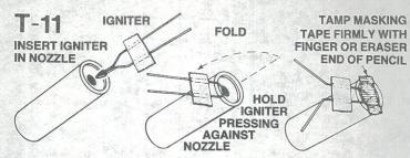
Select an engine and install an igniter as directed in the engine instructions. The engines recommended for use with this rocket are the A8-3, B4-4, B6-4, C5-3, and C6-3. Use an A8-3 for your first flight.
