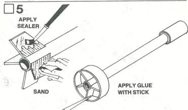
Do not proceed with this step until the glue reinforcements are <u>completely</u> dry. Apply a coat of sanding sealer to each fin. Let dry and sand with fine sandpaper. Repeat the sealing and sanding process until the grain is filled and the balsa looks and feels smooth.
