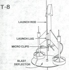
Slide the launch rod through rocket launch lug and place rocket on launch pad. Make sure the rocket slides freely on the launch rod. Clean the micro-clips and attach them to the igniter wires. Arrange the clips so they do not touch each other or the metal blast deflector. Attach clips as close to protective tape on igniter as possible.
