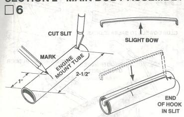
Mark the engine mount tube (part D) at 1" and 2-1/2" from one end. Cut a 1/8" long slit at the 2-1/2" mark. Gently bend the engine hook (part G) so that it bows upward very slightly in the middle. (Study the drawing.-Don't bend the wrong way.) Insert one end of the engine hook into the slit in the tube.
