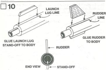
Sand the edges square on the remaining balsa parts. Lay the 2 small rectangles aside for use later. Glue the launch lug stand-off to the body as shown. Remember, the launch lug line is the one that is lined up with the engine hook. Next, glue the rudder to the opposite side of the body. Support the body as previously described and allow the glue to dry thoroughly.
