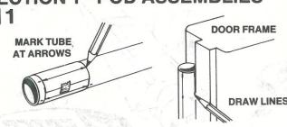
Cut out the BT-5 marking guide from page 5 of these instructions. Wrap the guide around one of the 5" long BT-5P body tubes (part A) and tape the ends together. Mark the tube at each of the arrow points. Remove the guide. Using the edge of a door frame as a guide, draw lines connecting the marks. Extend 3 lines about 2" from the end of the tube. Draw the fourth line the entire length of the tube. Repeat with the other BT-5P tube.
