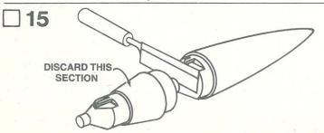
Separate the nose cone/adapter (part L) using either a sharp modeling knife or modeler's saw. Use the grooves molded into the part as cutting guide. Discard the adapter section, as it is not used.
