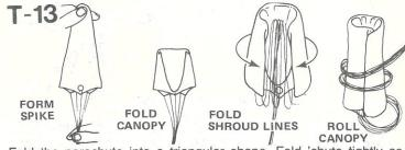
Fold the parachute into a triangular shape. Fold 'chute tightly as shown and wrap shroud lines around it. If 'chute is too large, unroll it and repack until it slides easily into rocket. A fit that is too tight may prevent parachute from ejecting properly.
