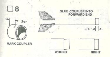
Mark the tube coupler (part H), 3/4" from one edge. Smear a band of glue inside the finned body tube about 1/4" from the forward end. Insert the coupler and push until the mark on the coupler is even with the end of the tube. Be sure the tube coupler is installed squarely as shown.
