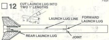
Cut the launch lug (part K) into two 1" lengths. Glue one of these lugs on the launch lug alignment line with its rear edge even with the line drawn around the tube as shown. Glue the remaining lug on the launch lug alignment line with its forward edge even with the joint where the two body tubes meet. Align the lugs straight on the body tube.
