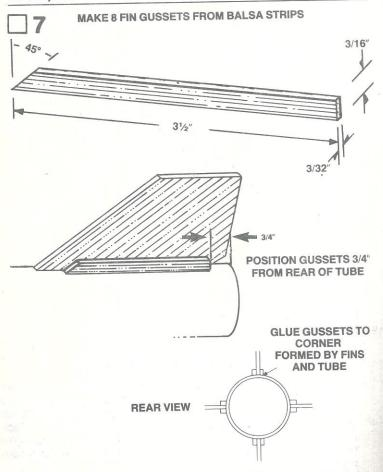
Cut 8 fin gussets from the 3 balsa strips (part G). Lightly sand all surfaces avoiding rounding any of the edges. Glue one gusset to each side of each fin where they touch the body tube. Use the illustrations as a guide for proper positioning.
