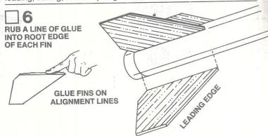
Rub a line of glue into the root edge of each fin and allow to dry. Glue the fins to the body tube on the fin alignment lines with the trailing edge of each fin even with the line drawn around the tube in step 4. The trailing edge of each fin should be on the 3/4" spacing line drawn around the body as shown.
