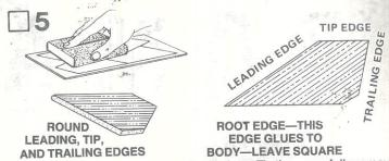
Fine sand the balsa fin die-cut sheets (part F), then carefully remove the fins from the sheets. Free the edges with a sharp knife. Sand the leading, trailing, and fin tip edges round. Sand the root edge square.
