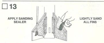
Proper application of sanding sealer makes the rocket look better and reduces drag so that the rocket will fly higher. However, this step is not essential to make a safe, attractive rocket. Apply a coat of sanding sealer to each fin and gusset. When sealer is dry, lightly sand all the sealed surfaces. Repeat sealing and sanding process until balsa grain is filled and smooth.
