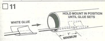
Smear glue over the back side of the shock cord mount as shown. Hold the mount so its narrow end enters the tube first and press it into place in the front of the body tube. Make sure the front of the mount is at least 1" or more from the tube end to allow for the nose cone. Hold the mount in place until the glue sets.
