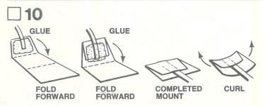
Cut out the shock cord mount from the display panel. Crease it on the dotted lines by folding. Spread glue on the first section (1) and lay the end of the shock cord (part J) into the glue. Fold over and apply glue to the back of the first section and the exposed part of Section (2). Lay the shock cord as shown and fold over again. Clamp the unit together with your fingers until the glue sets.
