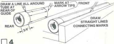
Cut out the body tube marking guide from the display panel. Wrap it around the body tube end which has the engine mount, 3/4" from the rear of the tube. Mark the tube at each arrow point. Draw a line completely around the tube at the rear of the guide as shown. Remove the guide and draw a straight line connecting each matching front and rear marks. (Use a ruler or other straight edge when drawing straight lines.) Extend the launch lug line the length of the tube.
