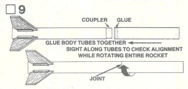
Smear a band of glue inside one end of  $12\frac{1}{2}$ " long body tube (part I) about  $1\frac{4}{4}$ " from the end. Slide this end of the tube over the coupler attached to the finned tube in one smooth movement. The edges of the two body tubes should touch all around. Sight along the tubes while rotating the rocket to be sure the alignment of the body tubes is perfectly straight.
