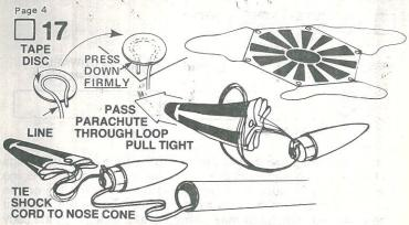
Cut out the parachute (part M) on its edge lines. Cut three 36" lengths of shroud line (part N). Attach the line ends to the top of the parachute with tape discs (part O) as shown. Pass the shroud line loops through the ring on the nose cone. Pass the parachute through the loop ends and draw the lines tight against the ring. Set the knot with a drop of glue. Tie the free end of the shock cord to the nose cone.
