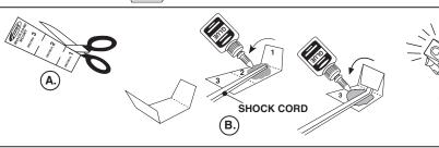
**A.** Apply glue to shock cord mount. **B.** Press mount into body tube about 25 mm (1") in from end of tube to allow for the nose cone.
