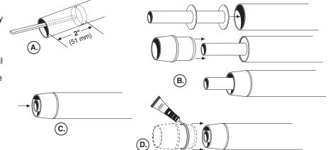
A. Cut out Tube Marking Guide from front of instructions. Wrap guide around the Body Tube and tape.
