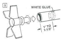
PUSH ENGINE MOUNT, WITH FIN UNIT/LOCK RING ASSEMBLY, INTO END OF TUBE.
