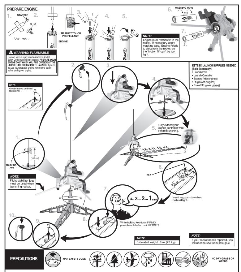
PRE-LAUNCH CHECK For safety, never launch a damaged rocket. Check the rocket's body, nose cone and fins. Also, check the engine mount, recovery system and launch lug(s).
