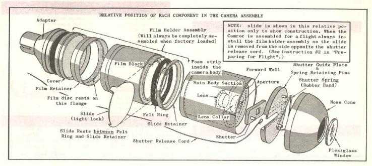
As soon as possible after recovery the tape around the joint between the film holder and the body of the camera should be peeled back just enough to uncover the slot for the slide. Immediately insert the slide all the way. The less time the Camroc spends out in the sun without the slide in place the better, since the chances of a ruined picture are reduced considerably when it is in place. (For additional protection, keep the camera shaded from the sun when the slide is being removed or re-
