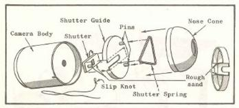
assembly into the front of the camera body. Center the slot of the shutter assembly on the small slot in the body so the shutter release cord comes straight through the body slot. Make sure the shutter guide assembly is seated into the camera body. Test the shutter. It should stick when the shutter is snapped.
