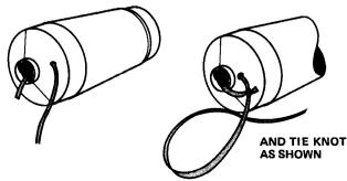
41 Tie one end of remaining shock cord (SC-2) to nose cone.
