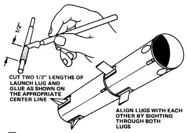
24 Using a dowel or stick for internal support, cut two 1/2" lengths of launch lug from the LL-3B and glue to body. Place launch lugs on launch lug center line and against retaining bands as shown.
