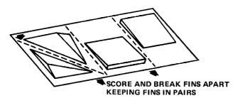
17 Use score and break method to separate the four fin halves on each plastic sheet. Keep fin halves in matched pairs. Each sheet contains parts for a complete upper and lower stage
