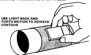
14 Wrap a sheet of sandpaper around body and sand bases of fin pads to match contour of body tube.
