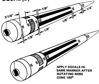
37 Apply twelve red 31's to nose cone as shown. Place six on each side. There should be three black stripes and two white stripes separating 31's applied in vertically striped area.
