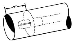
6 Mark the inside of the main body tube (BT-101LA) 3" from one end. Place engine mount/stuffer tube assembly inside main body tube with engine hook at the marked end of main body tube. Slide assembly until the rear centering ring is even with the 3" mark. Apply glue to ring/tube joints at both ends. After these joints are fully dry, apply a second coat of glue to ring/tube joints. These joints must be sealed properly to minimize loss of ejection gases.
