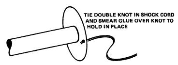
5 Tie a secure double knot at end of one of the shock cords (SC-2). Slip unknotted end through slit in forward centering ring and pull knot against ring. Apply a liberal coating of glue over the knot to hold it in place.
