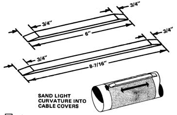
9 Cut cable cover stock into two lengths, one piece 6" long and the other 8-7/16" long. Taper ends as shown. Wrap a large piece of sandpaper around body and sand a slight curvature into bottom of cable covers.
