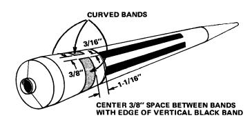
■ **36** Apply the three curved bands to nose cone as shown. There should be a 3/8" space between ends of bands and this space should be centered on edges of vertical black and white stripes. Smooth out all wrinkles and air bubbles and allow decals to dry.
