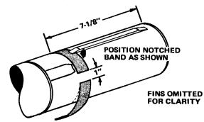
34 Remove 1" X 5.2" band with notch in one edge and apply to body upper stage. Center notch over lower end of cable cover. Apply a 1" X 5.2" band at same level with one inch between ends of bands.
