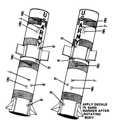
Apply red 31's and white decals in their locations as shown on the drawing above. Rotate body 180° and repeat application of decals as indicated. When all decals are completely dry, we recommend that the completed model be sprayed with Testor's "Dull-Cote" to protect the decals and model's finish.
