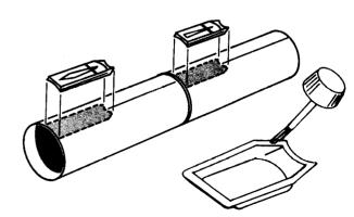
16 Working with only one pad at a time, carefully apply a thin layer of contact cement to all surfaces of fin pad which contact the body. Place pad in position on body while cement is still wet. Place it properly the first time to avoid smearing cement around. Use same method to cement remaining fin pads in place. If you have smeared cement on unwanted areas, use a pencil eraser to rub it off after it dries.
