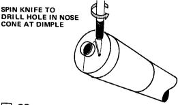
28 Use liquid plastic cement to cement top cone and base cone together. Use model knife to cut small hole (about 1/4" in diameter) in bottom of nose cone as shown.
