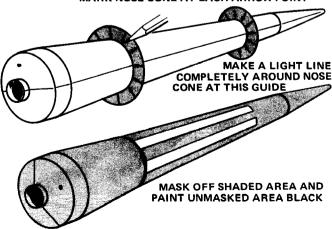
(SP-68) and place over nose cone as shown with one of the arrows on each guide lined up with one of the mold parting
