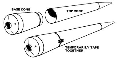
**26** Check fit of top cone (part number 71040) on base cone (part number 71041). If necessary, sand slightly for proper fit. Temporarily assemble nose cone, taping pieces together.
