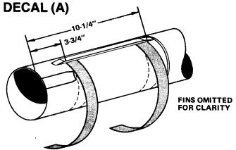
A Remove two longest bands from the orange decal sheet (A) and apply to lower stage body. Move decal into exact position and carefully blot away excess water with a soft cloth.
