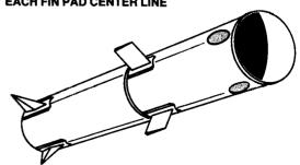
23 Place the three thrust reversal port covers (from watertransfer decal sheet (A)) on fin pad center lines 1/8" from forward end of body. Place them with their longest dimension running lengthwise on body.
