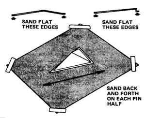
19 Tape a 8-1/2" X 11" sheet of 100 grit sandpaper to a flat work surface. Sand back of each fin half until the flange portion is about half of its original thickness. This will give a smooth fit between fin halves and a strong, neat joint when cemented together.
