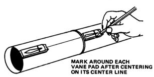
15 Place each fin pad in its proper place on the body and mark around it with a pencil. This will aid in proper placement when cementing in place. Be sure to center pads on their guide lines. The longer pads with diamond shaped fin outlines go at the rear of the body. The short pads with triangular fin outlines go against forward edge of rear retaining band.
