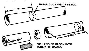
1 Mark engine casing (EC-6) 1/4" from one end. Use your finger or a stick to smear a band of glue inside engine mount/stuffer tube (BT-50L) about 2" from one end. Insert engine block (AR-2050) into end with glue. Use casing (EC-6) to push engine block into place (with the casing mark even with end of tube) with one smooth movement. Remove casing immediately.
