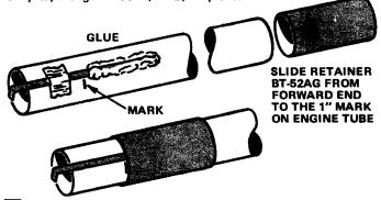
Apply a heavy line of glue on the engine hook from the 1" mark to the engine block end. Slip engine hook retainer (BT-52AG) onto forward end of stuffer tube and slide it back over engine hook to the 1" mark. Wipe away any excess glue and remove tape from engine hook.
