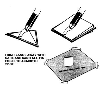
21 Use model knife or single edge razor blade to trim away most of the flange around each fin. Use sandpaper to trim to final size. Use fine sandpaper for final sanding on fin edges.
