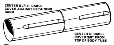
10 Glue 8-7/16" long cable cover in place with its upper end against lower retaining band. Glue 6" long cable cover in place with its upper end 3/8" below edge of body. Be sure cable covers are centered on their guide line.
