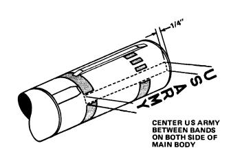
38 Apply "US ARMY" decals to body. Center decal on imaginary line between pin holes from step 25 and between self-adhesive bands.
