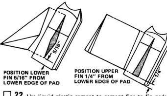
Use liquid plastic cement to cement fins to fin pads. Match bases of fins with fin outlines on fin pads. Lower stage fins are triangular with a diamond shaped base; upper stage fins are rectangular with a triangular shaped base.
