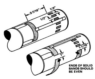
Apply the six 0.4" X 1" strips as shown. Apply remaining 1" X 5.2" band at same level with 1-1/16" between ends of bands. Blot away excess water when decal is in position.
