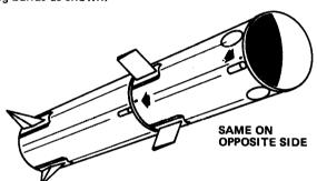
25 Use straight pin to put four small pinholes on the two charge retainer center lines, one on each line just below upper retaining band and one on each line just above lower retaining band. These holes are for later use in positioning decals.
