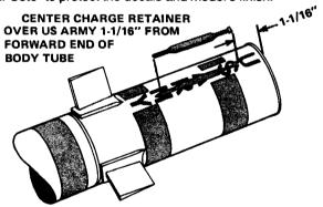
40 Use contact cement to attach both charge retainers to body. Be very careful not to smear cement on unwanted areas of body.
