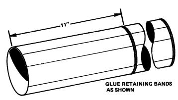
8 Cut retaining bands from pattern sheet and glue around body. Glue one with its top edge even with the 11" line and glue other with its top edge even with the front end of the body.
