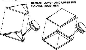
20 Be sure fin halves are arranged into matched sets. Work with only one set of fin halves at a time. Apply liquid plastic cement to flange surfaces on both fin halves and press
