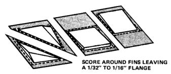
18 Use metal straight edge as a guide and trim fin halves (using score and break method), leaving a flange 1/32" to 1/16" wide around each fin half. Work carefully.
