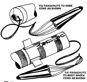
42 Assemble the two parachutes (PK-24A's) by directions on parachutes and tie one parachute to each shock cord (nose cone and body).
