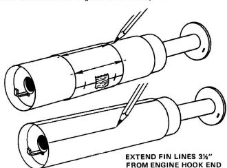
LI 8 Cut out fin spacing guide (part A). Wrap guide around the 8-1/2" long body tube (part C) and tape ends together with alignment marks matched. Mark body at each arrow point. Use a pencil because ink will show through paint. Remove spacing guide and connect each set of marks with a straight line. Fin lines should extend 3-1/2" from engine hook end of tube. The launch lug line should be extended to both ends of tube.
