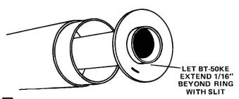
Glue centering ring (with slit in it) onto end of stuffer tube as shown. This ring was saved in step 4.
