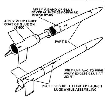
■ 16 Smear a band of glue inside part B as shown and apply a very light coat of glue on stage coupler. Being very careful to line up launch lugs on fin unit and forward tube, slide part B over centering ring and stage coupler. If glue squeezes from joint between body tubes, use a damp rag and wipe off excess glue immediately (be careful not to smear glue).
