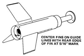
11 Mark each fin line 5/16" from rear of part C. Glue a fin on each fin line (centered on line) with rear edge of fin at 5/16" mark.
