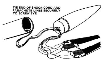
17 Remove nose cone from rocket and pull shock cord from stuffer tube (be sure that it comes out front end of tube). Tie end of shock cord to screw eye with a secure double knot.
