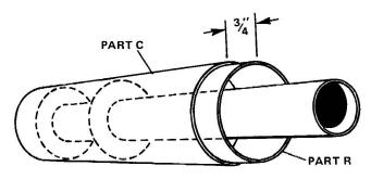
Glue stage coupler (part R) into forward end of part C. Part R should extend 3/4" beyond end of part C. Wipe off any glue on exposed portion of part R.
