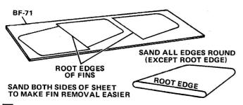
10 Lightly sand both sides of die-cut balsa fin sheet (part L) and remove fins. Gently sand all fin edges (except root edges) to airfoil shape shown.
