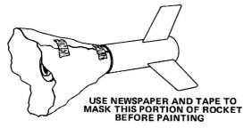
L 12 Use newspaper and masking tape to mask stage coupler and stuffer tube. Paint fin unit. Use Flat Black enamel spray for suggested paint pattern.
