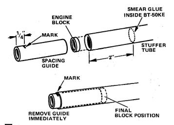
1 Mark engine block spacer (part S) 1/4" from one end. Use your finger or a stick to smear a band of glue inside stuffer tube (part D) about 2" from one end. Insert engine block (part F) into this end and use spacer to push engine block into place (with mark on spacer even with end of tube) with one smooth movement. Remove guide immediately.
