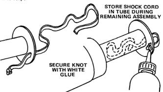
15 Tie a secure double knot at one end of shock cord (part J). Push unknotted end through slit in forward centering ring (from rear) and pull knot against ring. Apply a heavy coating of white glue over knot to hold it in place. Insert shock cord in stuffer tube to store it while continuing assembly.
