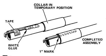
Apply a heavy line of glue on engine hook from slit to 1" mark. Slip engine hook retainer (part E) onto forward end of stuffer tube and slide it back over engine hook to the 1" mark. Wipe away any excess glue and remove tape from engine hook.
