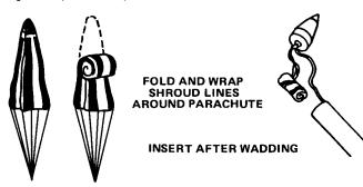
13 Fold the parachute into a triangular shape. Roll 'chute tightly as shown and wrap shroud lines around it. If 'chute is too large, unroll and repack until it slides easily into rocket. A very tight fit may prevent parachute from ejecting properly.
