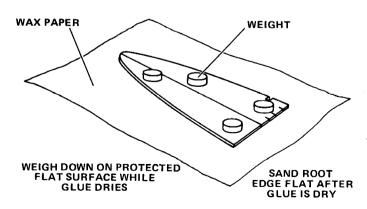
Garefully remove the parts from the die-cut balsa sheets (part J). The best method is to first sand both sides of each sheet smooth, then free the parts, where necessary, with a sharp knife. Glue the sails together as shown, making sure you match one notched and one unnotched half. Lay the sail assemblies flat on a piece of waxed paper and weight down to hold in position while the glue dries.
