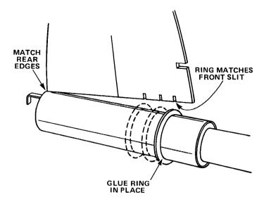
part K) on the reactor body using a sail for a guide. The ring should match the front slit on the sail when the rear of the sail is even with the rear of the reactor body. Glue the ring to the body in this position. A drop or two of glue is sufficient—do not over-glue. Use the sail to make sure the ring is correctly positioned all around the body. Slip the other two rings onto the reactor body in their approximate positions, but do not glue.
