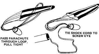
LJ 26 Cut out the parachute (part S) on its edge lines. Cut three 36" lengths of shroud line (part T). Attach line ends to top of parachute with tape discs (part U) as shown. Pass shroud line loops through screw eye. Pass parachute through loop ends and draw lines tight against screw eye. Set knot with a drop of glue. Tie free end of shock cord to screw eye.
