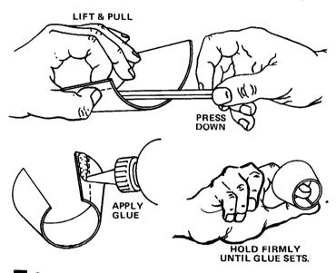
Pre-form the shroud (part C) by pulling it under a knife handle or pencil as shown. Pull the shroud under the handle or pencil and up at the same time. Do this several times until the cone can be formed easily. Apply glue to the tab on the cone and press into position exactly as shown. Hold it in place until the glue sets.
