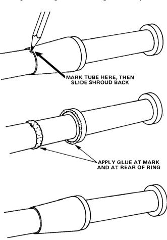
Slide the shroud onto the body and up against the first ring as shown. Mark the body where the end of the shroud touches it. Slide the shroud back and apply a line of glue around the body at the mark and around the ring where the shroud will touch. Slide the shroud back into position.
