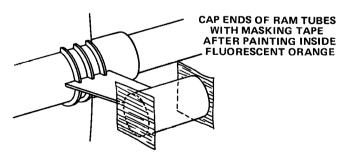
**27** Apply two or more coats of sanding sealer to balsa surfaces. Sand lightly with extra fine sandpaper between coats. Repeat until pores are filled and surfaces look and feel smooth. Paint the insides of the ram tubes white, followed when dry with a coat of bright fluorescent orange paint. Cap the ends of the ram tubes with masking tape and paint all other parts of the rocket flat black.
