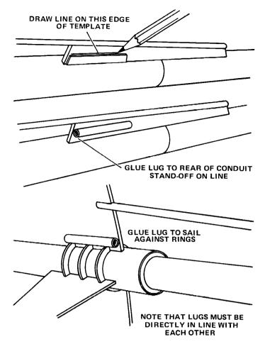
**20** Cut out the launch lug location template from the pattern sheet. Mark the lug location on the conduit stand-off on the same side as the antenna platform. Glue one launch lug (part O) to the conduit stand-off on this mark. Glue the other lug to the sail--against the radiator rings and directly in line with the first lug.
