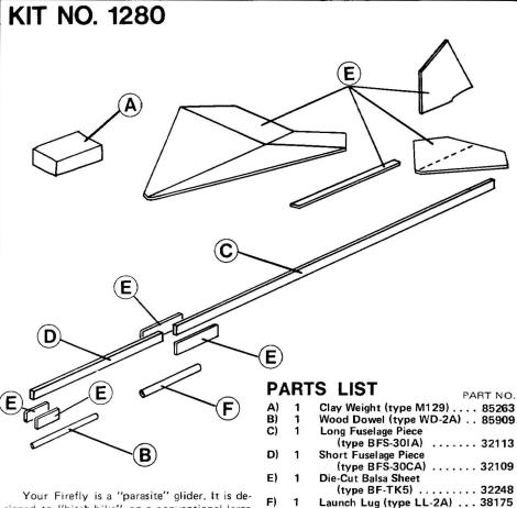
Your Firefly is a "parasite" glider. It is designed to "hitch-hike" on a conventional large model rocket on the upward flight, then glide back separately. A launch lug, taped to the side of the launch vehicle in the appropriate location, is generally the only modification required to adapt the launch vehicle to parasite operation.
