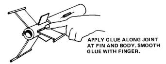
15 When the fin joints have dried, apply glue reinforcements to each main fin joint. Holding the fin mount assembly level, apply a narrow line of glue to both sides of each fin joint. Smooth out the glue with your finger. Keep the fin assembly level until the glue dries.
