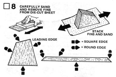
Fine-sand both sides of the balsa fin sheets (part I & J). Carefully remove the fins from the sheet using a sharp knife to cut free the corners and edges. Stack the rear fin set and sand as shown. Repeat the process with the forward fin set. Sand round each fin edge except the body edge. The body edge must be square.
