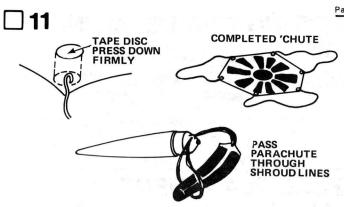
Cut out the parachute (part M) on its edge lines. Cut three 24" lengths of shroud line (part N). Attach line ends to the top of the parachute with tape discs (part O) as shown. Pass the shroud line loops through the eyelet on the nose cone. Pass the parachute through the loop ends and pull the lines tight against the eyelet. Set the knot with a drop of glue. Tie the free end of the shock cord to the eyelet to the eyelet with a double knot.
