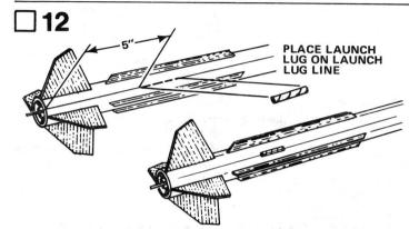
Glue the launch lug (part K) on the launch lug guide line so that the rear of the launch lug is 5" from the rear of the body tube. Align the launch lug straight along the body tube.
