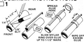
Mark across the engine mount tube (part A) 1/4" and 1-1/2" from one end as shown. Cut a 1/8" wide slit in the tube at the 1/4" mark. Apply glue from the slit to the 1-1/2" mark. Push one end of the engine holder (part B) into the slit and press the main part of the hook into the glue. Apply a thin layer of glue 1/4" wide around the tube to the rear of the 1-1/2" mark. Slide the retainer ring (part C) over the engine hook and the rear of the tube up to the 1-1/2" mark. Wipe off any excess glue.
