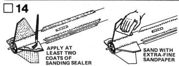
When all the glue on the model is dry, prepare the balsa fins for painting. Apply at least two coats of sanding sealer to all balsa surfaces. Let dry and sand thoroughly with the extra-fine grit sandpaper after each coat. Do this until all the tiny grain lines in the wood are filled and everything looks and feels smooth.
