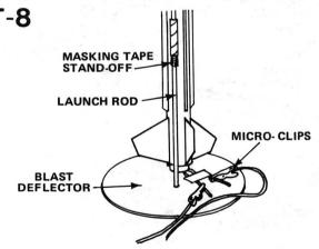
Slide launch rod through rocket launch lug and place rocket on launch pad. Make sure the rocket slides freely on the launch rod. Clean the micro-clips and attach them to the igniter wires. Arrange the clips so they do not touch each other or the metal blast deflector. Attach clips as close to engine as possible.
