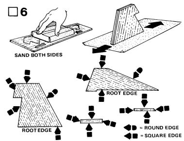
Fine-sand both sides of the balsa fin sheet (part G). Carefully remove the fins from the sheet using a sharp knife to cut free the corners and edges. Stack the large fins and the two pairs of small braces and sand as shown. Sand round only the leading edges of the three large fins. Both sets of braces remain square on all sides.
