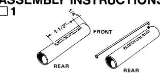
Cut a 1/8" wide slit in the engine mount tube (part A) 1/4" from one end as shown. Apply a 1-1/2" long line of glue to the tube as shown. Push one end of the engine hook (part B) into the slit and press the main part of the hook into the glue.
