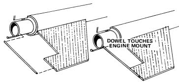
Cut the wooden dowels (part L) into four pieces, each 3" long. To make the laser, glue one dowel to each of the two balsa braces as
