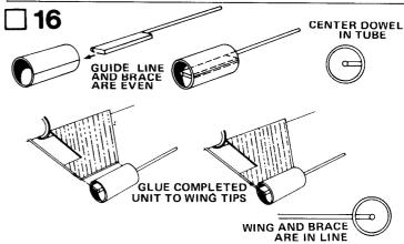
Using the guide line drawn in Step 11, glue the laser unit to the inside of the laser tube I so that each end is even with the guide line. Adjust the laser so that it is in the center of the tube. Glue the completed unit to the wing tip along the guide line. The balsa brace should look like a section of the wing as shown. Repeat for the other laser.
