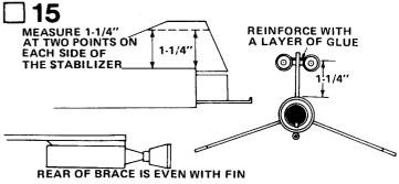
Measure 1-1/4" along the stabilizer from the body tube as shown. One measurement at the rear of the main body tube, another measurement as far forward as possible. Do this on both sides of the stabilizer. Draw a line between the two points. Glue the thrusters to the stabilizer along the line so that the rear of each brace is even with the rear of a stabilizer as shown. Once the glue is set, add a layer of glue to the brace connecting the stabilizer and the thruster
