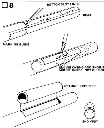
The object of this step is to cut a slot in the main body tube so that the  $5^{\prime\prime}$  long body tube will nest partially into the main tube. Study the drawings before beginning.
