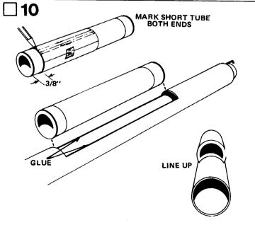
Mark the 5" body tube at a point 3/8" from EACH END. Wrap the marking guide around the tube and use one end as a guide to draw
