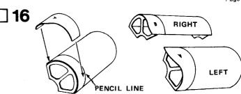
Cut shrouds A and B from the printed sheet and attach to the BT-60 units in a similar manner as you did in Step 14. Pre-curl the shrouds and glue to the tubes with the rear edge of the shrouds on the pencil lines (from Step 12). Note that there is a right unit and a left unit.
