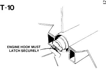
Insert engine into rocket engine mount. Engine hook must latch securely over end of the engine.
