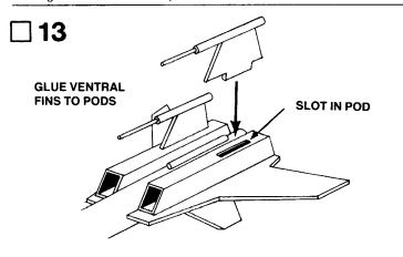
Apply glue to the root edges of the ventral fins and attach them to the bottoms of the engine pods as shown. Make sure the fins extend straight down from the pods. Allow glue to dry, then apply glue reinforcements to the joints.
