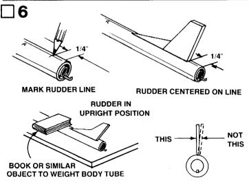
Place a mark on the rudder line 1/4" from the rear of the body tube. Apply a bead of glue to the root edge of the rudder. Hold it for a minute to allow the glue to become tacky, then attach the rudder to the body in the position shown. Make sure the rudder projects straight away from the body tube. Support the body with the rudder in an upright position. Allow the glue to dry completely before proceeding.
