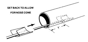
Use a finger or stick to apply glue to the inside of the front of the body tube, 1" to 2" from the front of the tube. Press the shock cord mount firmly into position in glue far enough from the front edge of the tube to allow clearance for the nose cone to fit into place. To insure a good bond use a stick or your finger to smear a film of glue over the mount and surrounding area in the body tube.
