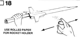
Paint the entire model gloss white. Follow instructions on the spray can for best results. We recommend spray enamel. Do not paint the model with lacquer paint. Shake can before spraying. Hold the can straight up and spray in long, smooth "strokes". Spray the model with several light, dry mist coats of paint to avoid "runs". Shake can periodically. Be sure paint is completely dry before applying decals.
