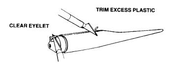
Trim or sand any excess plastic from around the sides of the nose cone (part J). Use a sharp knife to remove any excess plastic from the inside of the molded eyelet at the rear of the nose cone. Wash the nose cone with lukewarm soapy water, rinse well, and dry.
