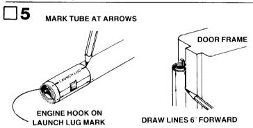
Cut out the tube marking guide from page 5 of the instruction sheet and wrap it around the rear of the body tube. Place the tube marking guide so that the engine hook is lined up with the launch lug line. Mark the body tube at each of the arrow points, write the letter "R" on the tube next to the marks for the rudder line. Remove the marking guide. Using a door frame as a guide, draw lines connecting each pair of marks. Extend the lines about 6" forward along the body tube.
