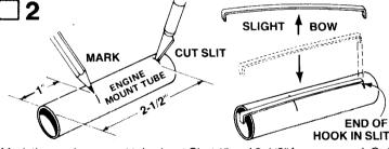
Mark the engine mount tube (part C) at 1" and 2-1/2" from one end. Cut a 1/8" long slit at the 2-1/2" mark. Gently bend the engine hook (part D) so that it bows upward very slightly in the middle. (Study the drawing.—Don't bend the wrong way.) Insert one end of the engine hook into the slit in the tube.
