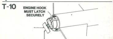
Insert engine into rocket engine mount. Engine hook must latch a ecurely over end of the engine.
