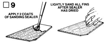
Apply a coat of sanding sealer to each fin. Apply sealer to all edges <u>except</u> the root edge. When sealer is dry, lightly sand all the sealed surfaces. Repeat sealing and sanding process until balsa grain no longer shows. Resand root edge, lightly, to remove any trace of sealer.
