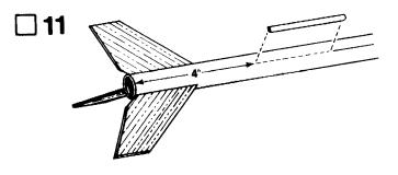
Glue launch lug (part I) to rocket body tube on the launch lug line. The rear of the launch lug should be 4" from the rear of the rocket body tube. Align the launch lug straight along the body.
