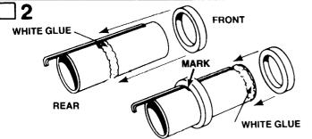
Apply a line of glue around the tube just forward of the 1-3/4" mark. Slide one of the adapter rings (part C) onto the tube from the forward end, over the engine hook, and up to the 1-3/4" mark. Apply a line of glue around the tube just forward of the engine hook. Slide the remaining adapter ring onto the forward end of the tube until it just touches the engine hook.
