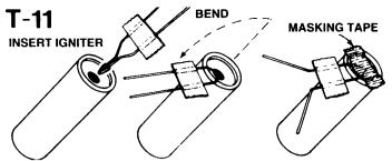
Select an engine and install an igniter as directed in the engine instructions. Use a D12-5 engine only.
