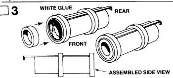
Smear a line of glue around the inside of the forward end of the engine mount tube and push the engine block (part D) in until it stops against the engine hook. Set the unit aside to dry.
