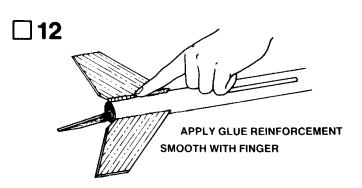
Apply glue reinforcements to each fin/body tube joint. Holding the model level, apply a narrow line of glue to both sides of each fin joint. Smooth out the glue with your finger. Apply glue reinforcement on both sides of launch lug. IMPORTANT—Keep the model level until the glue dries.
