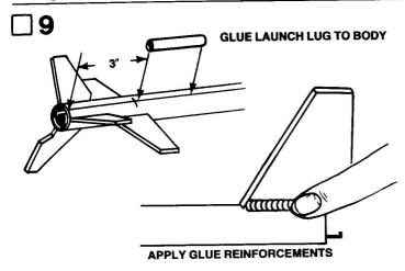
Place a mark on the launch lug line 3" from the rear of the body. Glue the launch lug (part G) in place, centered on the line, with the rear of the lug on the 3" mark. For added strength, all glue joints must be reinforced. Apply a bead of glue to both sides of the rudder-body tube joint. Pull your finger along the joint to smooth the glue into an even fillet. Repeat the procedure with the wing, fin, and launch lug joints. Lay the model in a horizontal position and allow the glue to dry.
