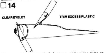
Trim or sand any excess plastic from around the sides of the nose cone. Use a sharp knife to remove any excess plastic from the inside of the molded eyelet at the rear of the nose cone. Wash the nose cone with lukewarm soapy water, rinse well, and dry.
