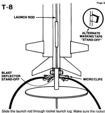
Slide the launch rod through rocket launch lug. Make sure the rocket slides freely on the launch rod. The rocket must be supported by a "stand-off" to keep the igniter wires from touching the metal blast deflector. If your launch system does not have a stand-off, wrap a piece of masking around the launch rod to support the rocket. Clean the micro-clips and attach them to the igniter wires. Arrange the clips so they do not touch each other or the metal blast deflector.
