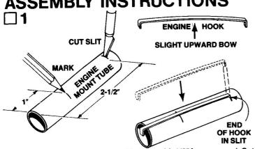
Mark the engine mount tube (part A) at 1" and 2-1/2" from one end. Cut 1/8" long slit at the 2-1/2" mark. Gently bend the engine hook (part B) so that it bows upward very slightly in the middle. (Study the drawing—Don't bend the wrong way.) Insert one end of the engine hook into the slit in the tube.
