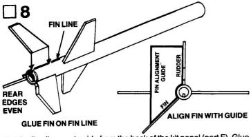
Cut the fin alignment guide from the back of the kit panel (part F). Glue a fin to the body as shown. Use the fin alignment guide to properly align the fin angle. Support as previously described while the glue dries. After the assembly has set for 5 minutes, re-check the alignment and, if necessary, adjust the fin. Repeat the procedure with the remaining fin.
