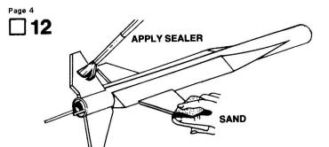
Apply a coat of sanding sealer to the wings, fin and rudder. When the sealer is dry, lightly sand the sealed parts with fine sandpaper. Repeat the sealing and sanding process until the balsa grain line is filled and the parts look and feel smooth. Lightly sand the glue joints on the cardstock fairings.
