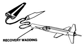
Pack 3 or 4 squares of loosely crumpled recovery wadding into the body tube. Usually this will fill the body tube for a distance equal to about 1-1/2 times its diameter.
