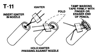
Select an engine and install an igniter as directed in the engine instructions. The engines recommended for use with this rocket are the A8-3, B4-4, B6-4, B8-5 or C6-5 made by Estes. Use an A8-3 engine for your first flight.
