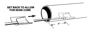
Use a finger or stick to apply glue to the inside of the front of the body tube, 1" to 2" from the front of the tube. Press the shock cord mount firmly into position in glue far enough from the front edge of the tube to allow clearance for the nose cone to fit into place. To insure a good bond use a stick or your finger to smear a film of glue over the mount and surrounding area in the body tube.
