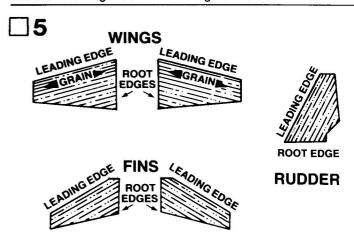
Lightly sand both sides of the die-cut balsa sheet (part E). Free the parts by running a knife along the die-cut lines. Sand all edges square. Sort and identify the parts as shown above. "Leading edge" is the edge that faces forward and "root edge" is the edge that is glued to the body tube.
