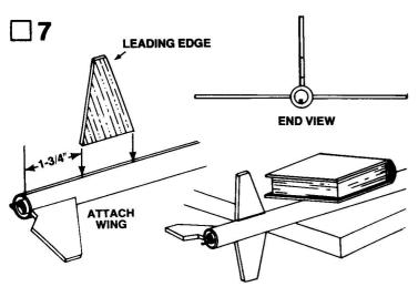
Place a mark on each wing line 1-3/4" from the rear of the body. Before gluing the wings, make sure you have them oriented as shown. The grain of the wood is parallel with the leading edges. Glue one wing in place, centered on the line, with the rear edge on the 1-3/4" mark. Adjust the wing so it extends from the body at a 90° angle to the rudder. Support as shown while the glue dries. Attach the remaining wing in the same manner.
