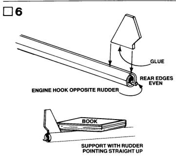
Apply a bead of glue to the root edge of the rudder. Attach it to the body, centered on the rudder line as shown. Make sure the rudder extends straight from the body. Set the body on a table with the rudder pointing straight up. Lay a book or similar object on the front of the body so it won't roll. Allow the glue to dry.
