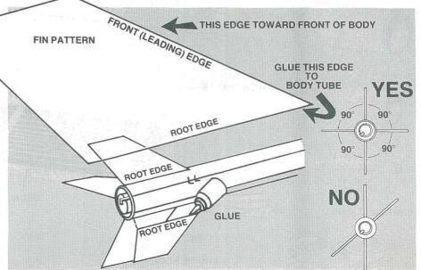
Glue launch lug straight on launch lug line 43/4" from rear of tube.
