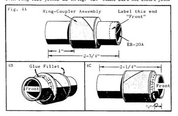
is well covered, wipe off any excess glue with your finger, and set the unit aside to dry completely. Next mark the 2-1 4" long engine holder tubes 1/4" from one end and glue the remaining two adapters in place as shown in fig. 4C. Set these aside to dry completely.
