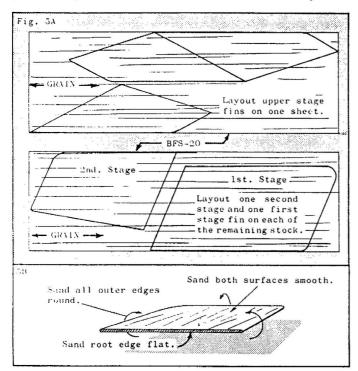
Cut out the fins with a sharp modeling knife or single edge razor blade. Sand the sides of the fins until smooth. Sand until smooth and round all edges except the root edge (the edge which will be attached to the body). Sand the root edge so it is square and flat.
