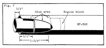
$\square$  (8) Mark the remaining two engine mounts 1/4" from their ends on the side that projects farthest from the adapter. Apply glue to the inside of one of the 2-3/4" long booster body tubes over an area 3/4" to 1-3/4" from one end and slide an engine mount unit into the tube. Position it as shown in fig. 8, with the
