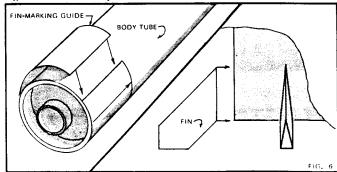
Cut out the fin marking guide (part G) and wrap it around the rear of the body tube. Mark the body tube at the points of the arrows. (Be sure the points are located over valleys in the cornigations.) Remove the guide and extend the mark up the body about 2". Spread glue on the root of one of the fins and carefully position it on one of the fin lines. Line up the fin by sighting down the tube. Repeat this step with the other three fins.
