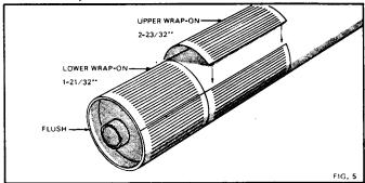
Roll the lower wrap-on (part F) around the tube. you have the wrap-on around the tube, line up the lower edge of the wrap-on with the lower end of the tube and draw a line on the tube around the upper edge of the wrap-on. Remove the wrap-on, spread a thin film of glue around the tube and roll the wrap-on back into place. The upper wrap-on is applied in the same manner as the lower one. Make sure the edges of the wrap-ons are tightly together and the end joints are in line.
