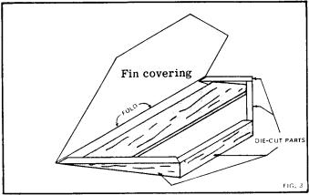
Cut the fin coverings from the pattern sheet. the coverings so that the word "Fold" is toward the inside. Punch out the die-cut fin framework pieces (part O) and sand slightly if needed to the proper size as snown on the pattern card (part G) or as shown in fig. 3. Then assemble as shown above.
