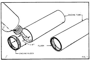
Glue the engine block (part C) into one end of the engine holder tube (part B). To do this, spread glue around the inside of one end of the engine tube to cover about 1/4". Slide the engine block into this end of the tube until it is flush with the end as shown in the illustration above.
