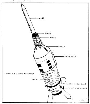
11. Apply a light coat of sanding sealer to all exposed balsa parts. When the sealer is dry, sand the parts lightly (but thoroughly). Apply a second coat of sealer let dry and sand some more. Repeat this until the pores in the wood are filled, then give the model at least one base coat of white paint. Follow with aluminum, black and the decals as shown fig. 11.
