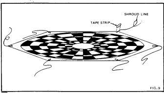
9. Cut out the parachute (part H) on its edge lines as indicated on the plastic. Cut six 18" lengths of shroud line cord (part I) and attach one shroud line to each point of the parachute with a tape strip (part J) as shown above. Tie the free ends of the lines together in a loop. Tie the end of the shock cord into this loop.
