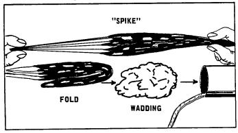
— 13— Hold the parachute between two fingers at its center and pass the other hand down it to form a "spike" shape as shown. Fold the "spike" into three sections Wrap two squares of wadding over the end of the parachute after it is folded, ready to be packed into the body tube. This gives the chute extra protection. Insert the shock cord and shroud lines into the body and place the parachute in on top. Slide the capsule into place.
