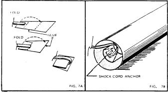
7. Cut out the shock cord mount from the pattern sheet and assemble it with one shock cord (part K) as shown in fig. 7A. Spread glue over a 1" square area on the inside of the body tube, at least 1-1/2" in from the front end of the tube. Lay the shock cord mount onto the glue and press it down into the shape of the tube. After the glue has set a thin layer of glue may be spread over the shock cord mount.
