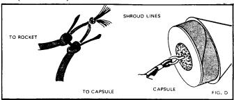
D) After capsule assembly is completed, tie one end of the remaining shock cord (part K) of the vehicle kit to the screw eye at the base of the capsule. Tie the other end to the loop in the parachute shroud lines as shown.
