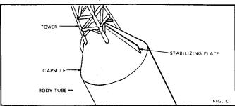
C) Capsule Assembly Step 14. After completing this step, cut out the stabilizing plates from the pattern sheet (vehicle kit part G) and glue them in place as shown in the capsule assembly illustration above.
