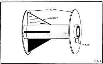
2. Punch out the two RA-2070 rings (part E). Glue one ring on each end of the engine tube about 1/8" in from each end. Punch out the four engine mount gussets from the die-cut balsa (part O) and glue them into place as shown in fig. 2. After the glue has dried, run a fillet of glue along all joints. Set this assembly aside to dry thoroughly.
