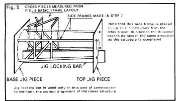
members in the drawing, then measure each piece and glue it in place as you did in step 7. When dry, remove the structure from the jig, turn the remaining side up, reassemble the jig and repeat the first two parts of this step. After the structure is completely dry, disassemble the jig from the structure and save the base and top jig pieces for use in the next steps.
