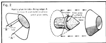
with the printed side to the inside. Slip the completed shroud over the capsule nose cone. It should seat against the shoulder of the cone, exposing about 1/16" of the flat area indicated.
