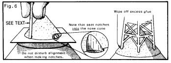
dowel or a 1/16" drill bit. Apply a drop of glue to each notch and fit the base legs of the tower structure into place. Wipe off any excess glue and let the assembly dry completely.
