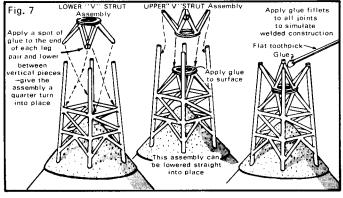
☐ 13. Apply a thin line of glue to the ring surface and a drop of glue to each leg joint of the upper "V" strut assembly. Slip this
