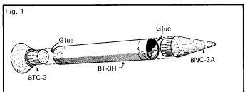
Apply glue just inside the other end of the escape motor tube and slip the tail cone into place as shown in fig. 1.
