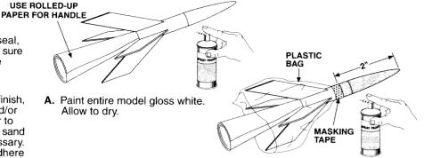
B. Mask off back end 2" from tip of nose cone & paint front end light blue or a bright color. Allow to dry.
