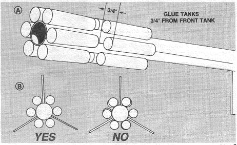
$(\mathbf{A})$ **APPLY THIN LINE OF WHITE** GLUE TO ALL WOOD/TUBE JOINTS, THEN SMOOTH OUT WITH FINGER
