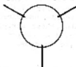
two fins. Do not set the rocket on the fins until the glue is fairly dry.
