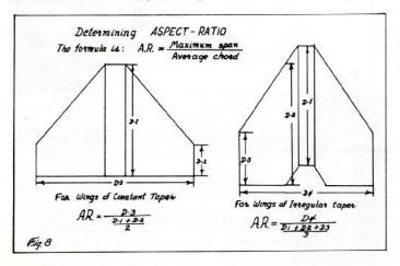
Also of importance is the effect of acceleration during boost. A one-ounce model's wings may weigh 23 times their normal weight for a short time during boost. For this reason, wings should be kept as light as possible consistent with adequate aerodynamic strength. Also, wings which have their CG closer to the body tube, or with low aspect ratios, will be more resistant to being torn loose from the body tube by acceleration forces.
