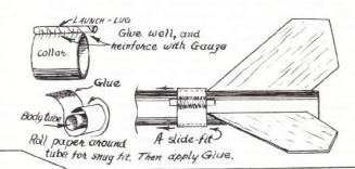
808 FLINT, Shawnee Mission, Kansas suggests a clean and easy way to hold a rocket off the wiring during countdown, if the fins do not hold rockets-end off of the launch-pad.
