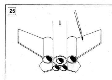
Apply sanding sealer to all the fins and sand with fine sandpaper. Repeat until all the grain is filled.
